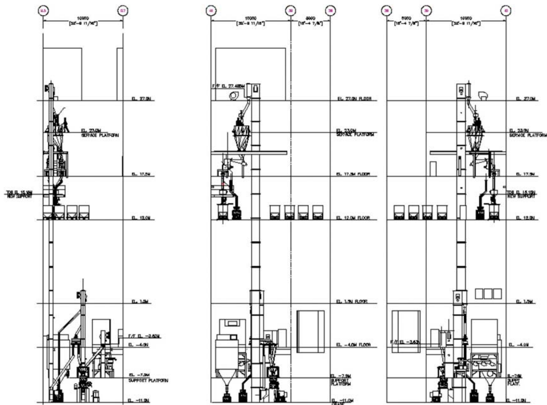
An orthographic drawing generated from the three-dimensional model representing three different elevation views of the equipment layout in a multifloor building.
