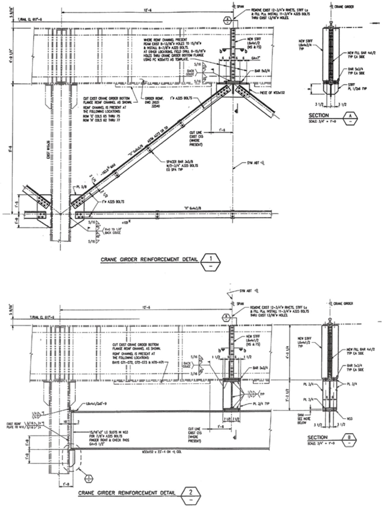
25' 0" crane girder reinforcement details.
