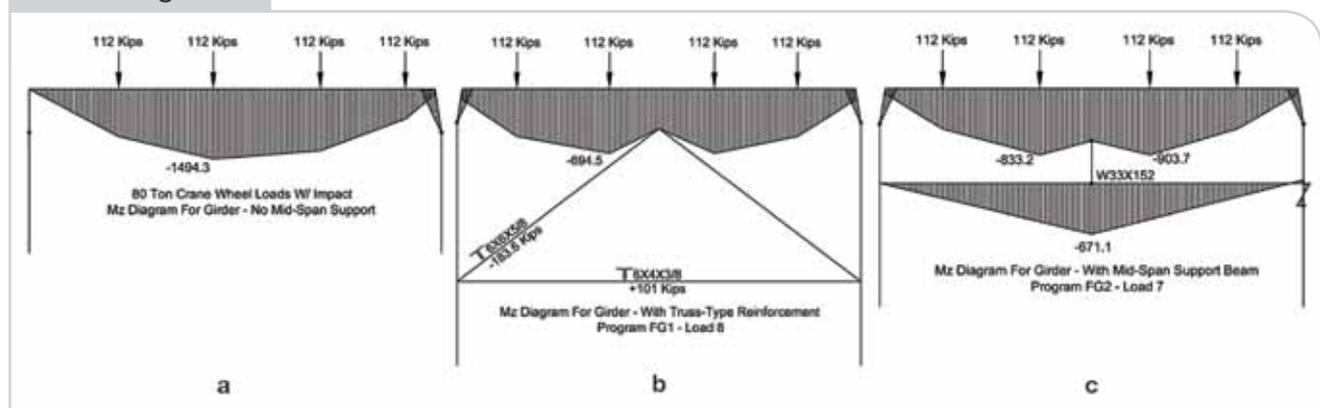
25' 0" crane girder reinforcement.
