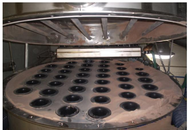
***This dust-collector tubesheet is leaking, allowing dust to pass from the dirty side below the tubesheet to the clean side above.***
