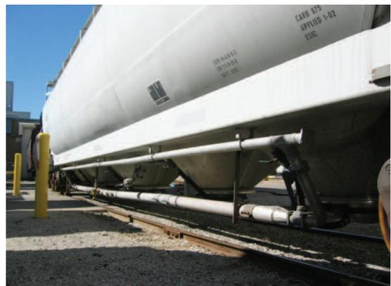
**When receiving material deliveries by rail car, ensure that all components of the rail car's pneumatic piping are present and in working order.**
