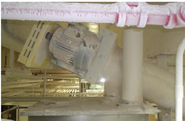
***Fugitive dust settled on high surfaces and pipes can be disturbed by an initial dust explosion in a vessel and create a combustible atmosphere for subsequent, larger explosions.***
